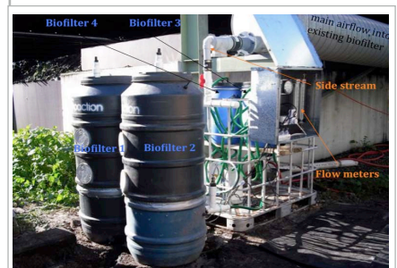
Figure 1 - Pilot test biofilters were placed at the inflow manifold feeding the primary biofilter at the RRRC
